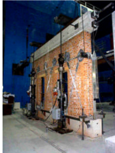
Figure 6: Full scale Model and SMAs based protection system
