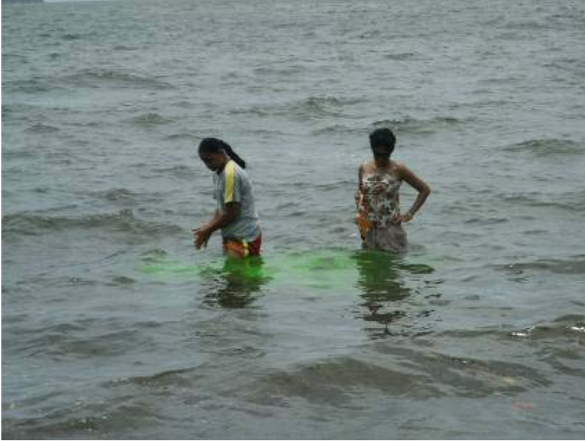
Measuring longshore currents, Suva Point, December 2005
