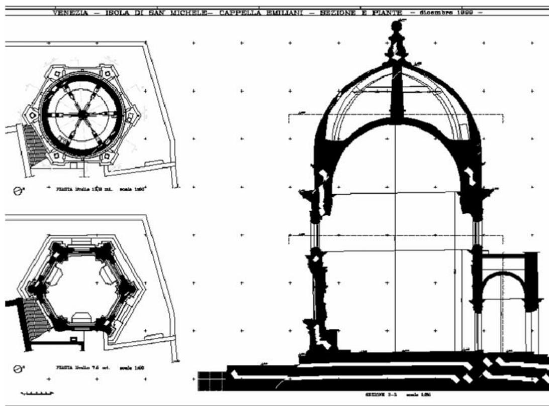
Fig. 6 - Ground plans of the Cappella Emiliana at two levels, and the main section (Drawing SAT Survey 1999).
