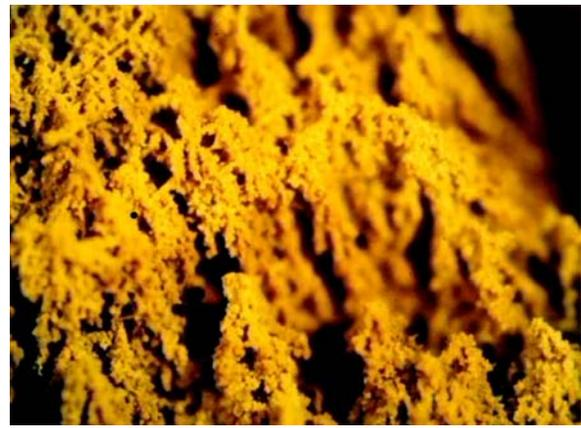
**Figure 6.** Goethe is an iron bearing oxide mineral occurring inside the rusticle structure.
