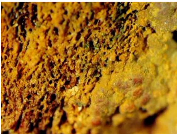
**Figure 5.** Lepidocrocite is an iron oxyhydroxide mineral occurring on the outside of the rusticle structure.
