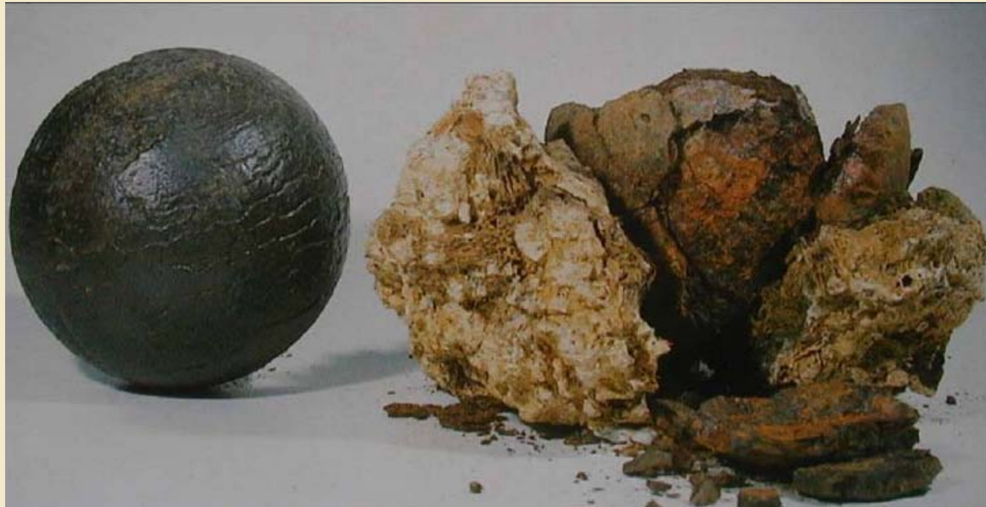
On the right an unconserved cannonball taken by looters from the Mary Rose , United Kingdom. On the left a cannonball from the same wreck, but which has been treated scientifically © Mary Rose Trust.
