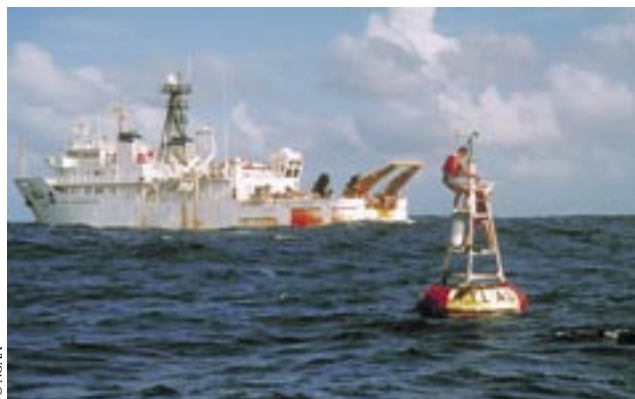
One of 70 fixed moorings in the tropical Pacific which monitor and forecast El Niño events within the global ocean observing system. The last El Niño event occurred in 2002–2003
