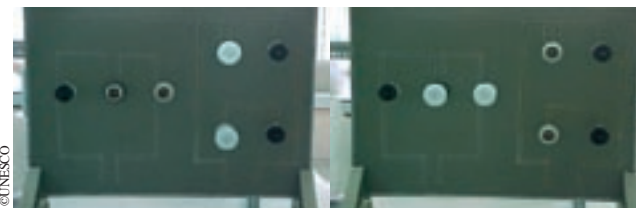
A demonstration of an electric circuit in series or in parallel can be constructed using a wooden board, electric bulbs, batteries and a switch. The apparatus can be used as an interactive demonstration in a lecture. By comparing the brightness of the bulbs connected in series or in parallel, students can see for themselves the difference between series and parallel circuits in terms of current and voltage, and the effect of switching the circuit on or off. This demonstration gives the student a real experience of electric circuits beyond the blind note-taking and copying of diagrams
