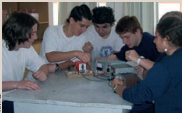
Here, pupils at the Instituto Ariel Hebreo Uruguayo are using an ammeter and a voltmeter to observe the changes in current and voltage in a simple DC-powered electric circuit
