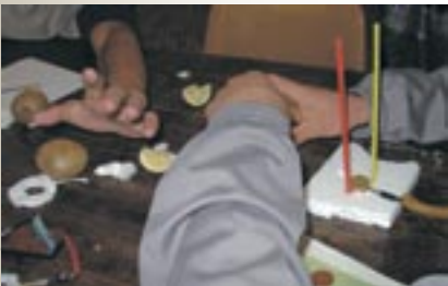
These children in Bologna, Italy, are building a Voltaic battery using coins, lemons and oranges. Citrus fruits have been chosen because the acidity of their juice makes them an excellent electrolyte (i.e. a very good conductor of electricity)
