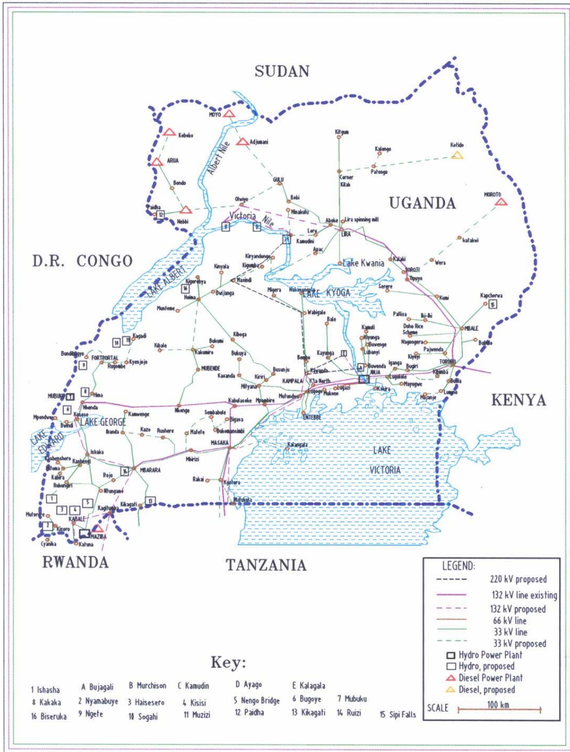
Figure 8.2 - Existing Electricity Grid and the Planned Extensions
